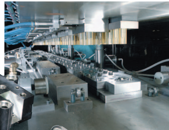
Friction Stir Welding uses a rotary dowel to join pieces with minimal influence on the material's properties. The joints are strong, homogeneous and porous-free.
