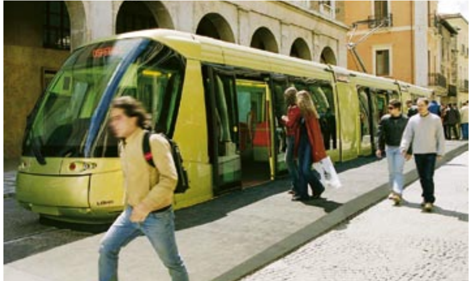
The tram's pneumatic tyres ensure a quiet ride.
