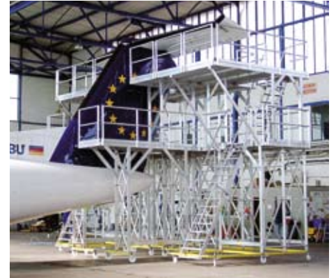
Stairways for maintaining aircraft.
