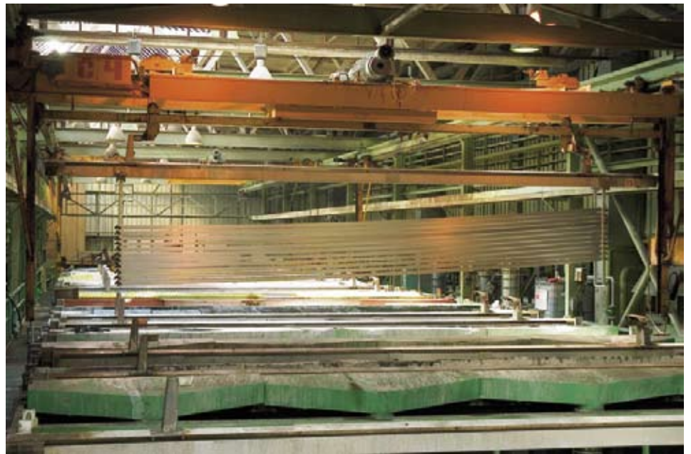
Anodising at Alufinal’s pressing plant in Ziar nad Hronom.
