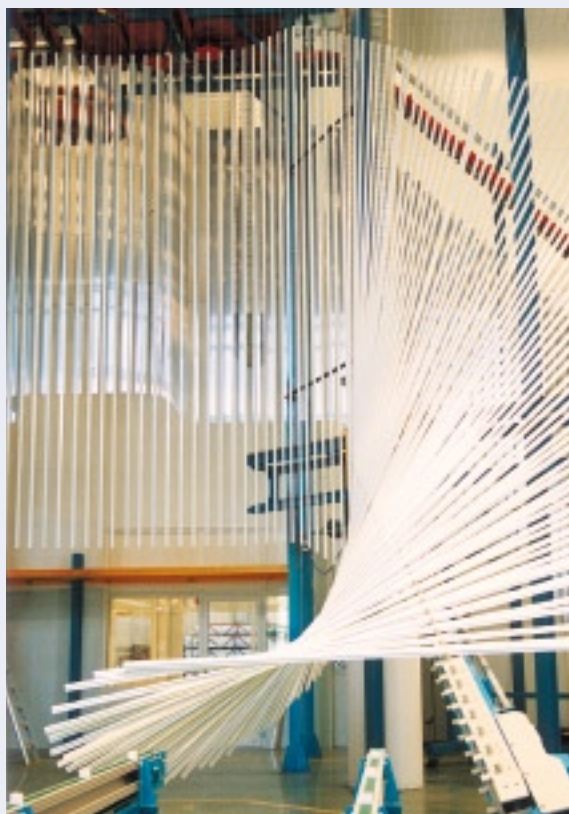
Vertical powder coating line.
