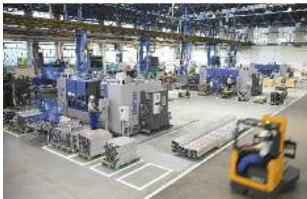
The Hungarian branch of Sapa manufactures its aluminium profiles on seven presses that create aluminium profiles from 80 g to 20 kg per running meter
