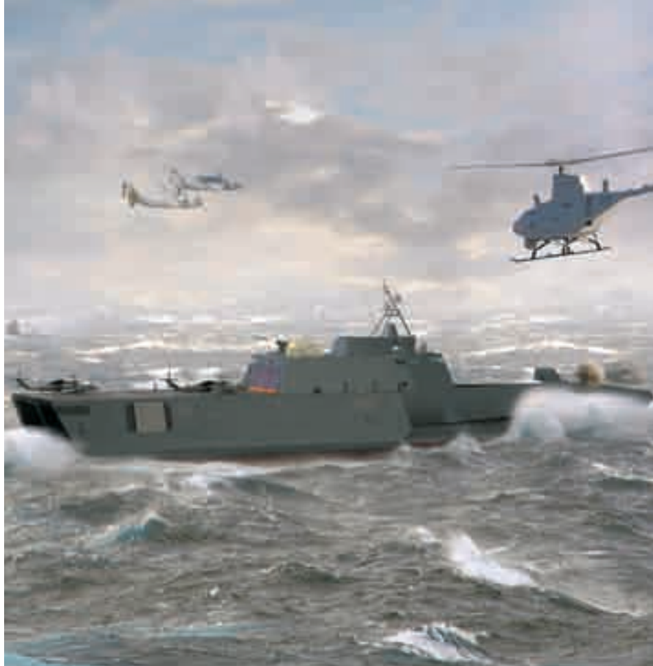
The Littoral Combat Ship is designed as a trimaran to withstand rough weather.
