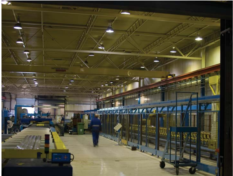
A view from the new Presezzi press with the double puller and flying saw on the right and cooling tables forward and to the left
