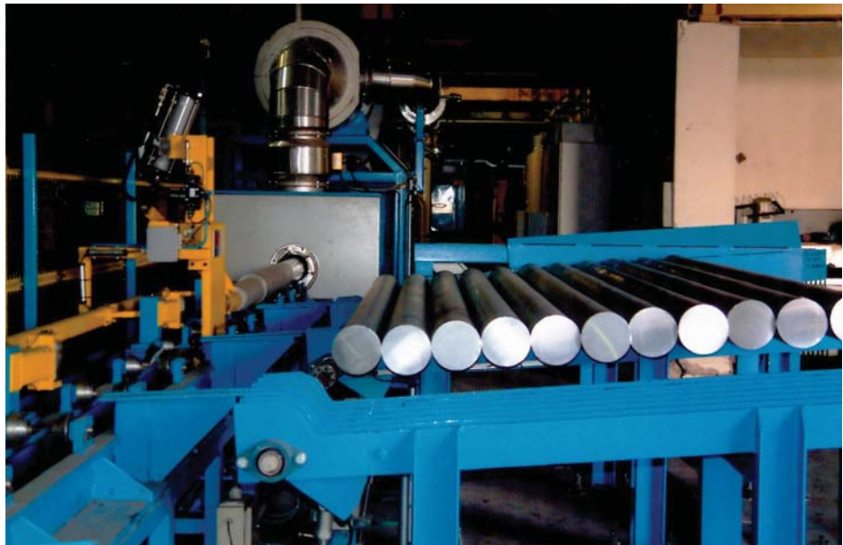
Billets entering the gas-fired heater serving the Presezzi press
