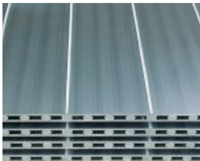
Panels for multi-plate freezer designed for fish industry: After joining the joint is milled. This gives a completely smooth surface easy to keep clean. The repeatability applies to all variables: the structure of the joint, its strength, leakproofness and panel levelness.
