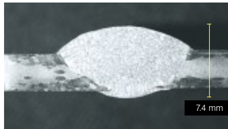
The MIG weld builds up. The filler material has a different chemical composition compared to the parent material.
