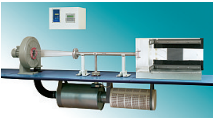
The wind tunnel makes it possible to verify calculations carried out using RapidCool and/or CFD analysis, and hence check the actual performance of the cooling device.
