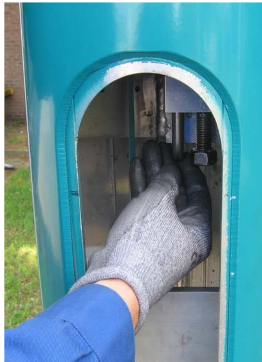
Pic. 16 Lock the column by pushing the pin up. Put handle of the pin in the "parking position".
