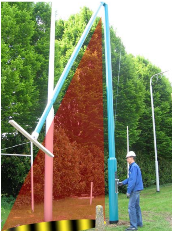
Pic.11 Note: Don't stand between the column and arm during operation.
