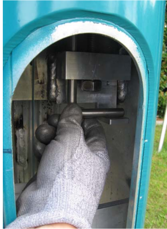
Pic. 18 Turn the handle of the pin' to the right, so it lays on the brace.
