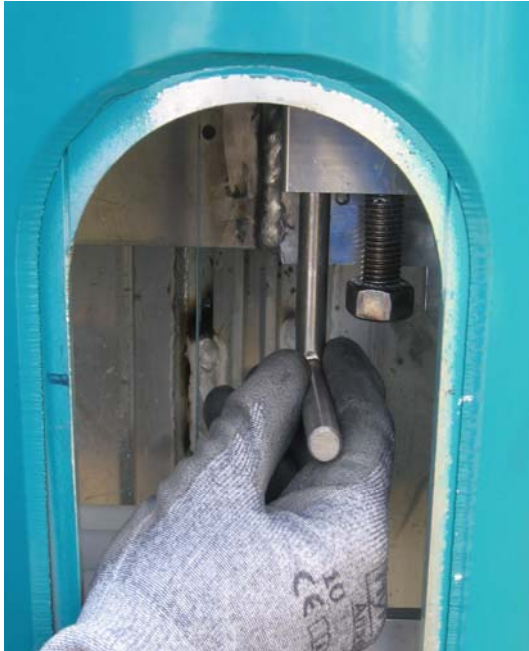
Pic.05 By pulling the pin down the hinge column will be unlocked.
