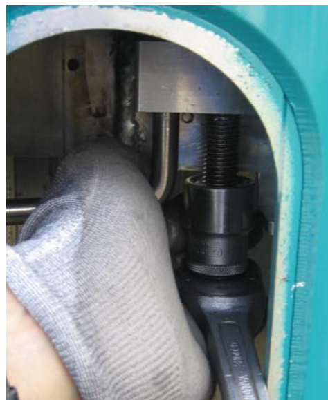
Pic.04 Unscrew the locking bolt using a tool (dimension across flats-24 mm), so it lays free on the brace.
